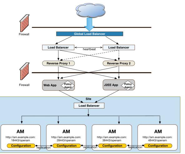
Site Deployment With a Single Load Balancer
