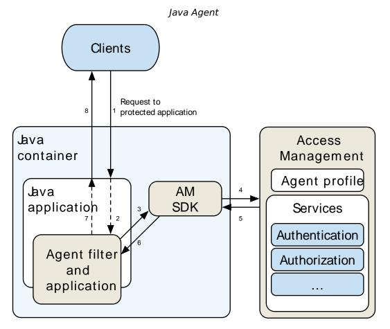
The figure represents the agent filter (configured in the protected Java application) and the agent application (deployed in the Java container) in the same box as a simplification.
