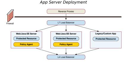
When the client sends an access request to a resource, the web or Java agent redirects the client to an authentication login page. Upon successful authentication, the web or Java agent forwards the request via the load balancer to one of the AM servers.
