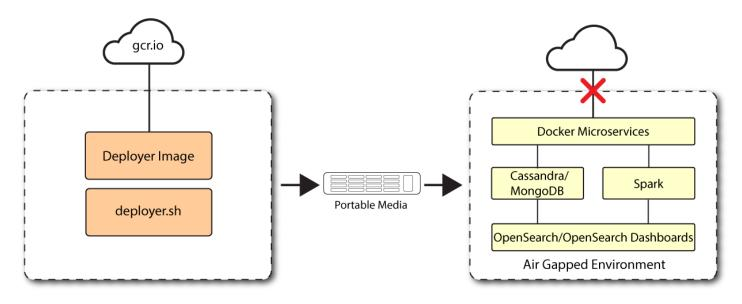
Figure 1. A single-node air-gapped target deployment.
