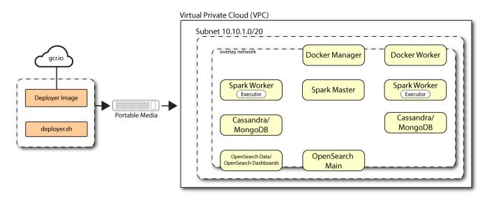
Figure 4. A multi-node air-gapped target deployment.
