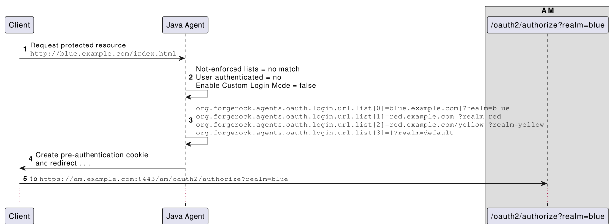
Figure 3. Data flow for default login redirect mode, where the user authenticates to a subrealm based on the request domain
