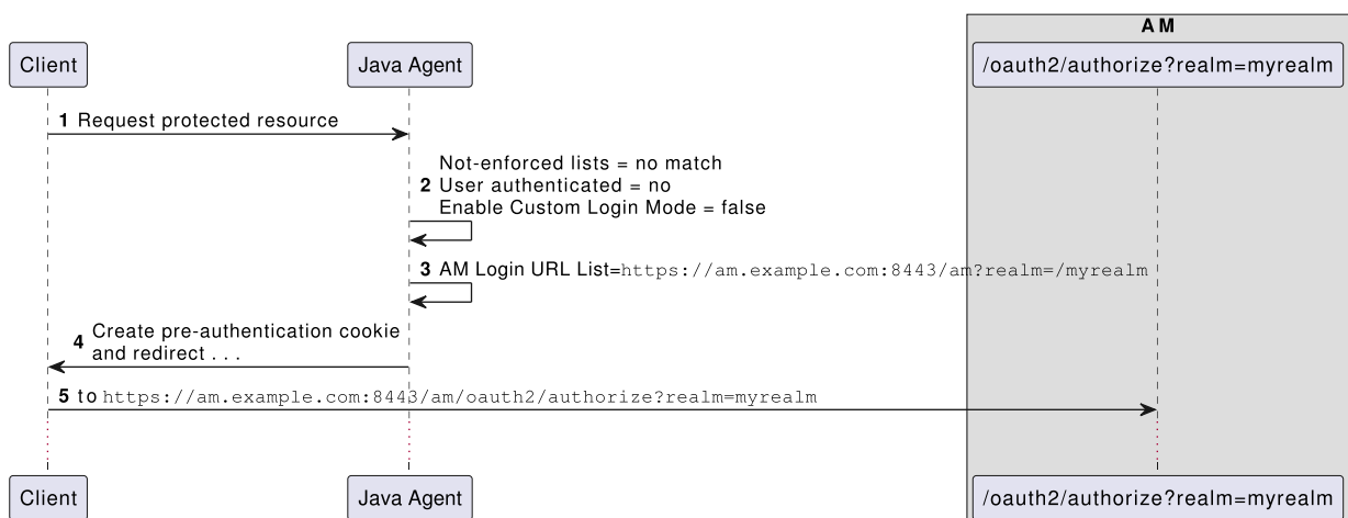
Figure 2. Data flow for default login redirect mode, where the user authenticates to a subrealm
