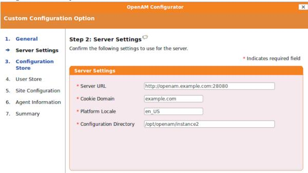
4. Click on Add to Existing Deployment?. Enter the Server URL of the first instance, for example <a href="http://openam.example.com:18080/openam">http://openam.example.com:18080/openam</a>. You should be able to accept the default settings once your Server URL has been verified.
