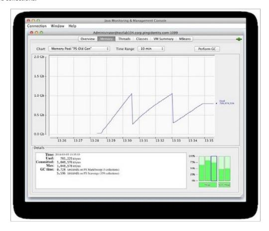
When a heap is sized inadequately, the Old Generation runs out of space.
