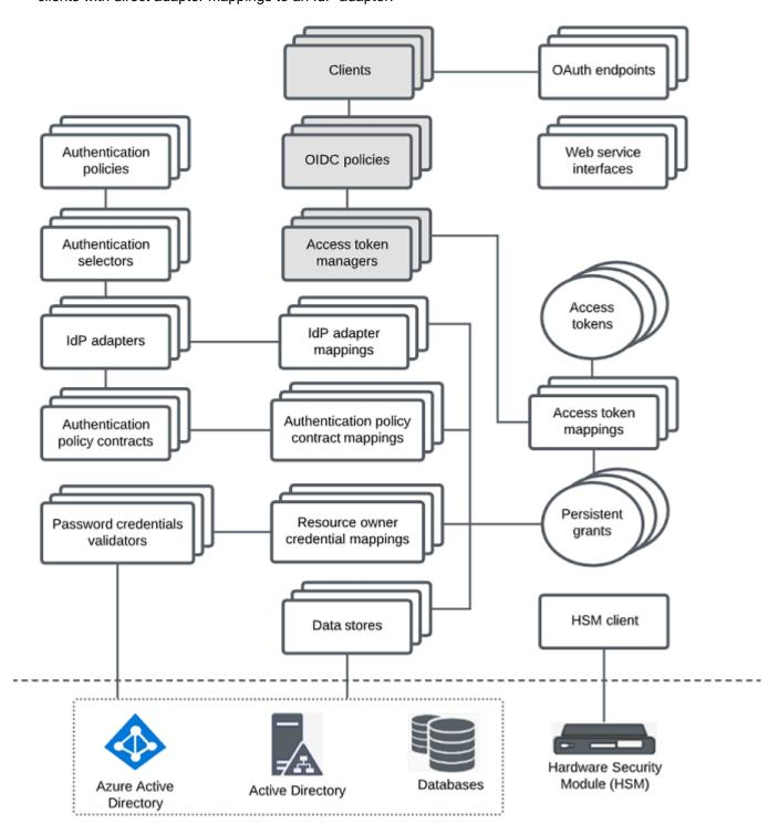
This diagram shows which PingFederate components are used to authenticate a SAML connection. PingCentral currently only orchestrates the PingFederate IdP connection, which is shaded in the diagram.
