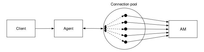
The following image shows the flow of information when a request is treated in a connection pool:
