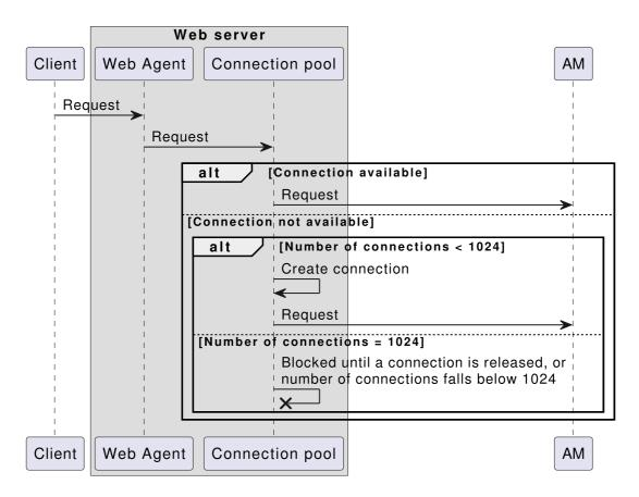
When a client makes a request, the agent intercepts the request and uses the connection pool to connect to AM. If a connection is available, the agent uses that connection. The client is unaware of the connection reuse.
