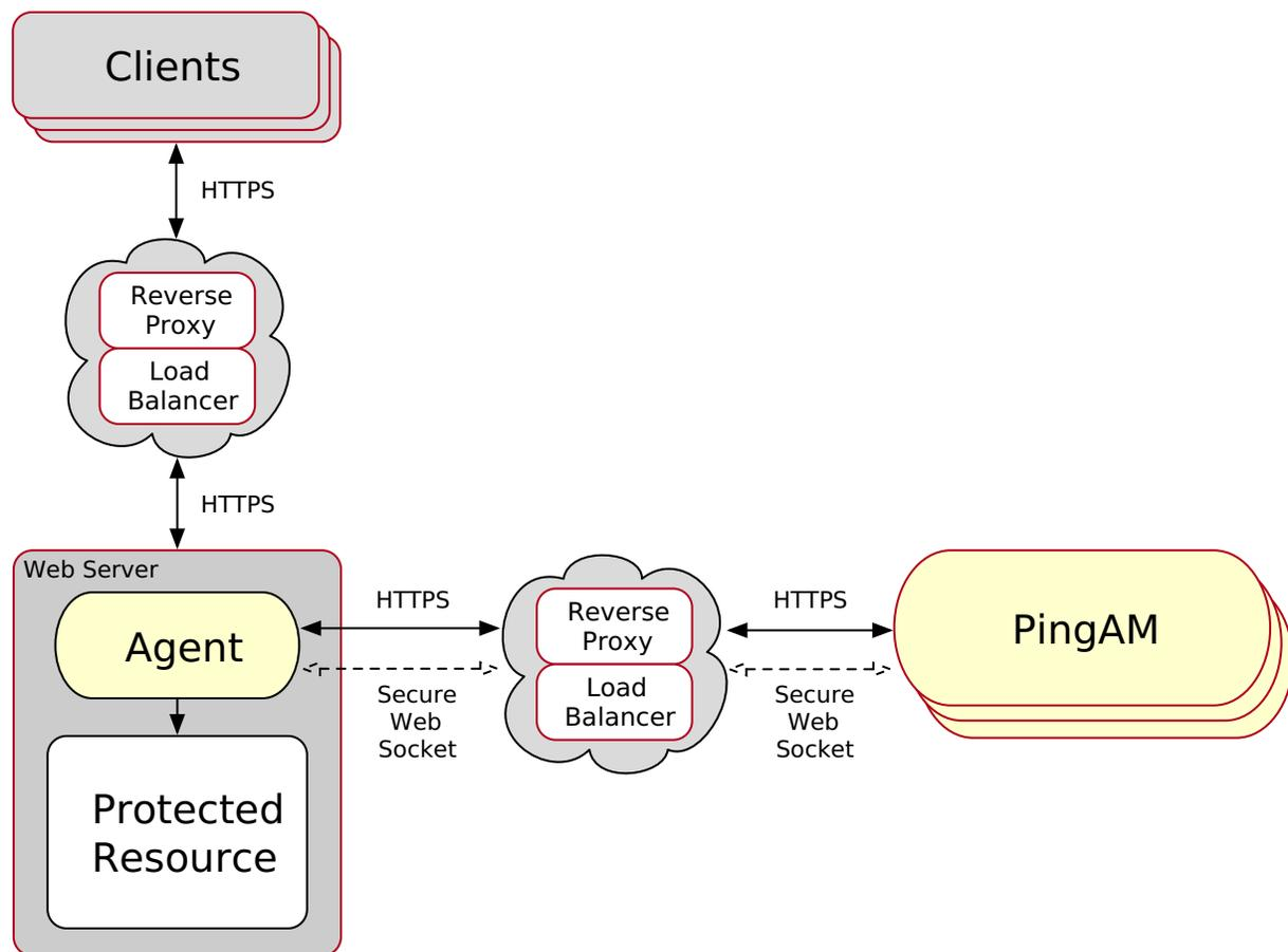
Figure 1. Environments with load balancers and reverse proxies
