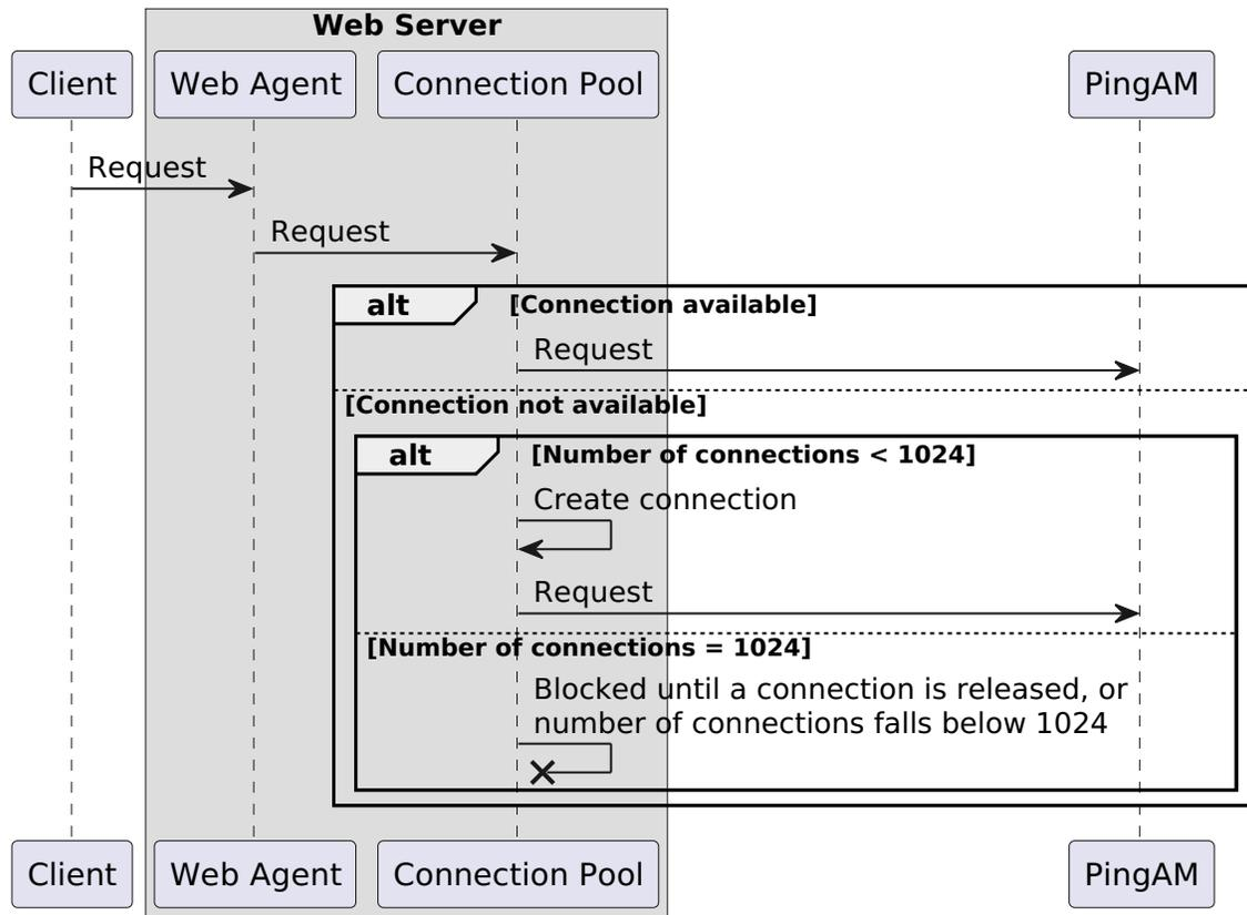
When a client makes a request, the agent intercepts the request and uses the connection pool to connect to AM. If a connection is available, the agent uses that connection. The client is unaware of the connection reuse.
