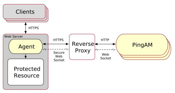
Figure 1. Apache HTTP Server reverse proxy configured between the agent and AM
